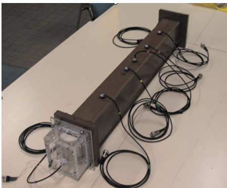
FIG. 5. (Color online) Measurement tube in the radiation configuration.
